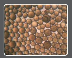
Fine mesh resin has an average bead size that is 23% smaller than standard mesh resin. With smaller beads, the ion exchange process happens more quickly. The result is less salt, less water, and less time is needed versus standard mesh for the same capacity.
