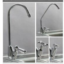
A multiple combination tap offering three different handles and two different spouts giving six combinations in all. The tap incorporates 1/4 turn, ceramic disc technology. Complete with 3/8"JG straight coupler. For use with 3/8" drinking line.
