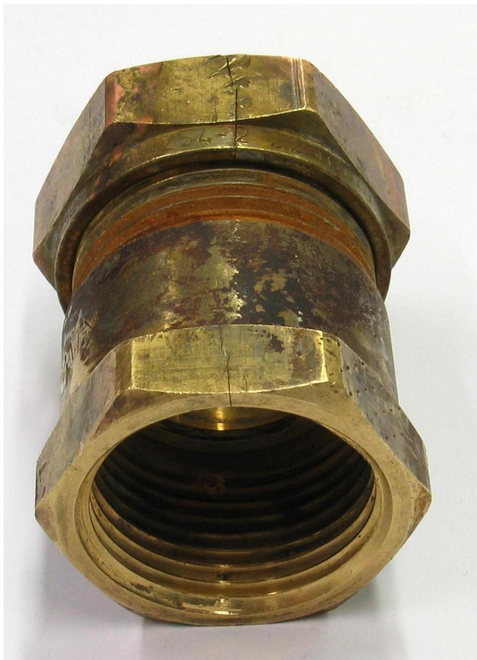
Figure 7 Stress corrosion cracking in a brass fitting.
