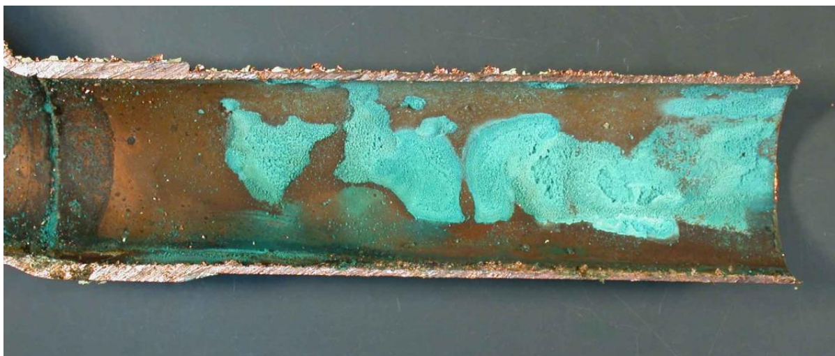
Figure 5a Irregular carbonate patina giving rise to blue water.
