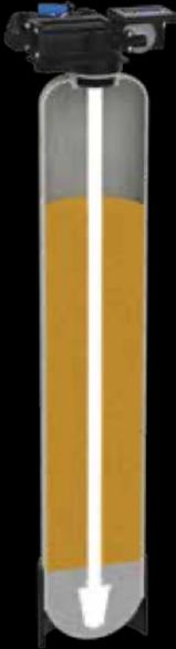
Conventional water treatment units have a design flaw that leads to water channeling or tunneling. The result is wasted media.
