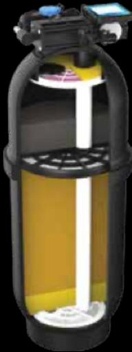
The WaterMax® is engineered with a baffle and distribution screens that distribute the water evenly through the tank to prevent water channeling.
