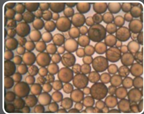
Fine mesh resin has an average bead size that is 23% smaller than standard mesh resin. With smaller beads, the ion exchange process happens more quickly. The result is less salt, less water, and less time is needed versus standard mesh for the same capacity.
